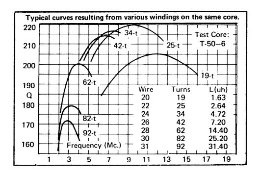
The above chart shows typical Q curves resulting from a number of various windings on the same toroidal core.
